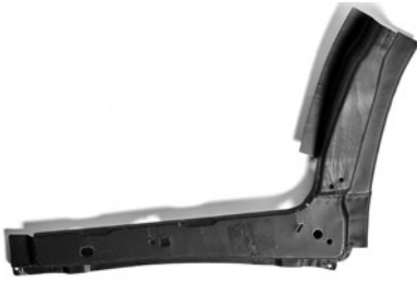
25-09-04-9 Inner Sill L/H 25-09-04-10 Inner Sill R/H
